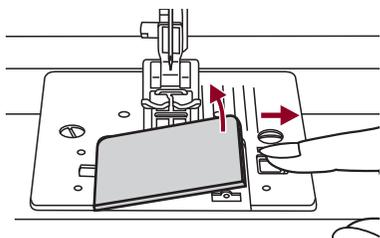
Remove the needle plate cover and bobbin.
