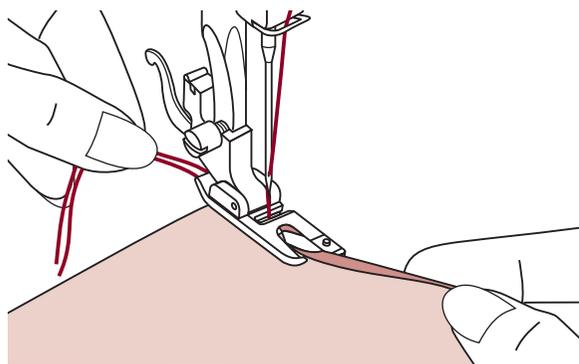
Insert the fabric fold into the spiral opening of hemmer foot. Move fabric back and forth until the fold forms a scroll shape.
