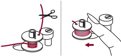
8. After the bobbin has wound a few turns stop the machine and cut the thread near the hole of the bobbin. Continue filling the bobbin until it is full. The motor stops automatically when the bobbin is full. Stop the machine. Push the bobbin winder spindle to left.
