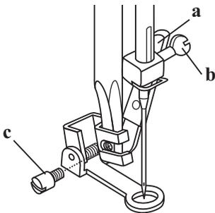
Remove the presser foot holder, and attach the darning foot to the presser foot holder bar.
