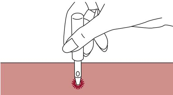
Make a hole at the center using an eyelet punch.
