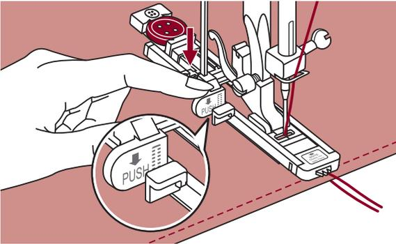
Pull the buttonhole lever all the way down and position it behind the bracket on the buttonhole foot.
