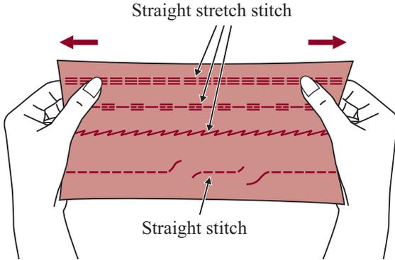
It assures you of a stitch that is strong and flexible and will give with the fabric without breaking. Good for easy to ravel and knit fabrics. It is good for joining durable fabric such as denims.
