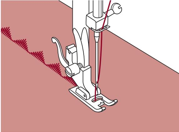
Use the satin stitch foot for satin stitching and sewing decorative stitches. This foot has a full indentation on the underside to allow easy sewing over the thickness of the stitches formed by closely spaced zigzag stitches, and even feeding of the fabric.
