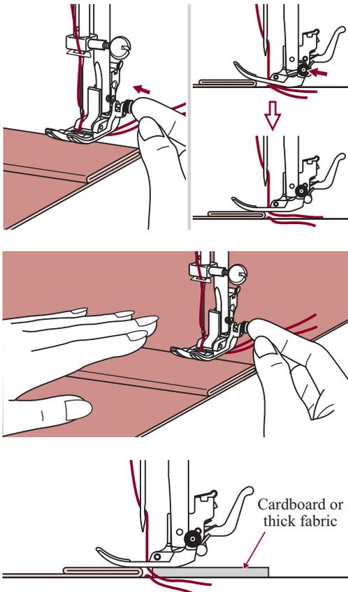
You also can place another piece of fabric with the same thickness at the back of the seam. Or support the presser foot while feeding by hand and sewing toward the folded side.
