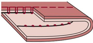
Thread tension is too loose for straight stitch sewing. Turn dial to higher number.
