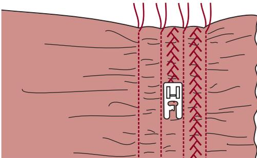
Reduce the tension, if necessary and sew decorative pattern stitches between the straight seams.
