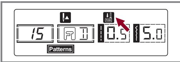
➔ **Please Note:** When you select any buttonhole pattern, LCD screen will be demonstrated the figure "👇", it is to remind you to lower the buttonhole lever.
