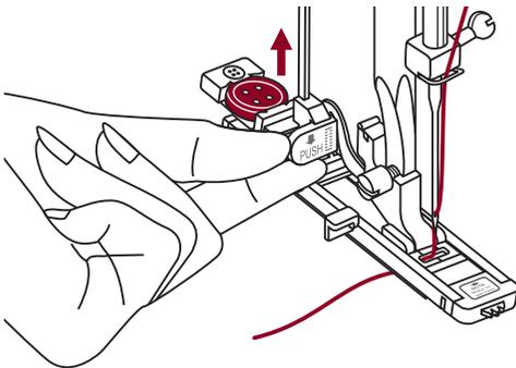
Buttonholes are sewn from the front of the presser foot to the back, as shown.
