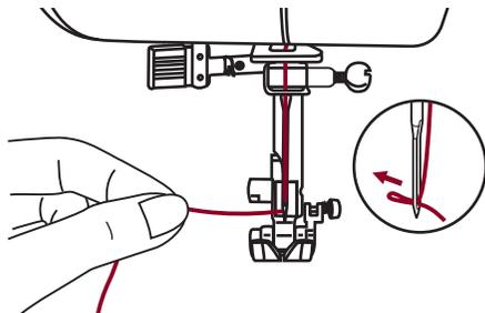
Hold the thread loosely and release the lever slowly. The hook will turn and pass the thread through the needle eye forming a loop.
