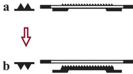
Move the drop feed control to "▼" to lower the feed dogs.
