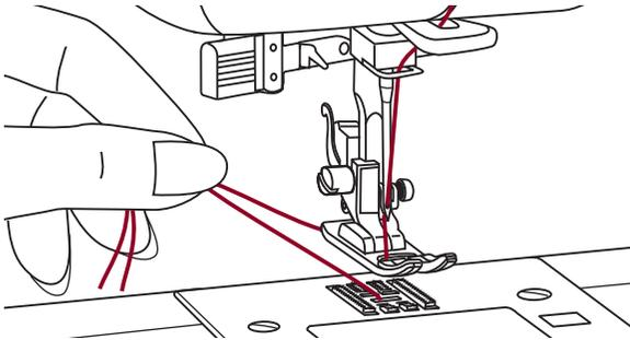
3. Pull both threads to the back under the presser foot.
