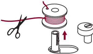
9. Cut the thread and then remove the bobbin.
