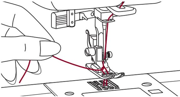
2. Gently pull on the upper thread to bring the bobbin thread up through the needle plate hole. The bobbin thread will come up in a loop.
