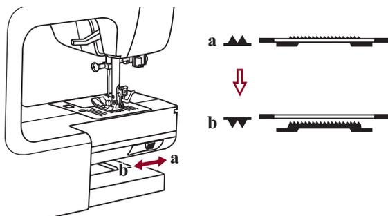
Sliding the lever to the "▼" (b) will lower the feed dog, for example during button sewing. If you wish to continue sewing normally, slide the lever to the "▲" (a) in order to raise the feed dogs.
