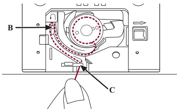
Pull the thread at the arrow markings into the stitch plate thread guide from (B) to (C).
