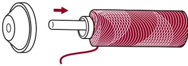
2. Snap the thread into the thread guide.
