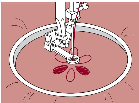
Secure with a reinforcement stitches at the end by press Auto-lock button.
