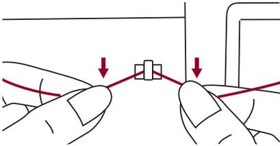
3. Wind the thread contrary clockwise around the bobbin winder tension discs.
