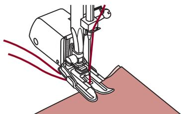
Draw the bobbin thread up and place both the bobbin thread and the needle thread behind the walking foot attachment.
