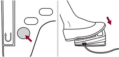
7. Press on the foot control or the Start/stop button to start winding the bobbin.
