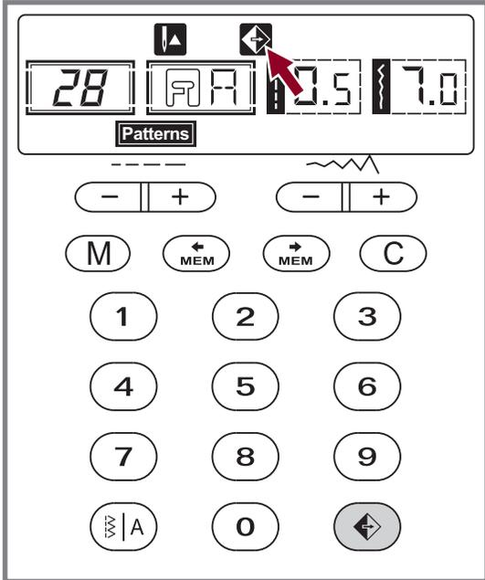
Pressing the mirror button. LCD will display the mirror function and the machine will sew the reflected pattern until you press the mirror button again.
