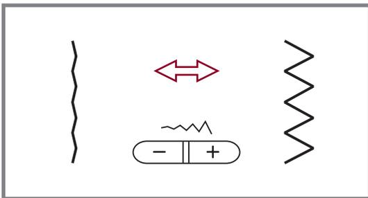
For a narrower stitch, press the "-" button (left). For a wider stitch, press the "+" button (right).
