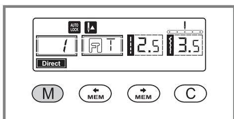
Press the "M" button to leave the memory mode and return to the Direct mode.
