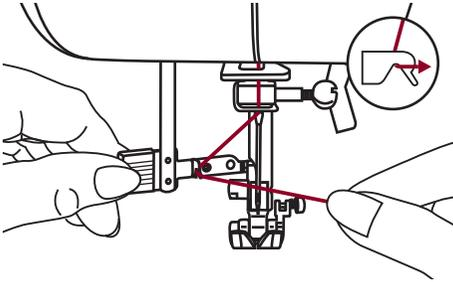
**Raise the needle to its highest position and lower the presser foot.**
