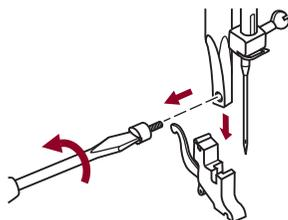
Remove the presser foot holder by unscrewing (counterclockwise) the presser bar attaching screw.
