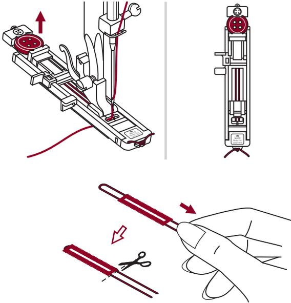
Attach the buttonhole foot and hook the gimp thread onto the back of the presser foot.
