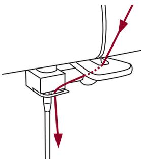
7. Pass the thread behind the flat, horizontal thread guide. Guide the thread through the wire loop. Pull the end of the thread through the needle from front to rear, and pull out about 10 cm of thread. Use the needle threader to thread the needle. (On the next page.)
