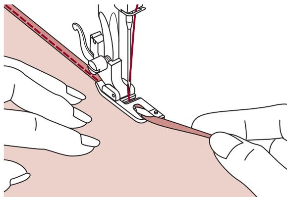
Lower the presser foot and start sewing slowly guiding the raw edge of the fabric in front of the hemmer foot evenly into the scroll of the foot.
