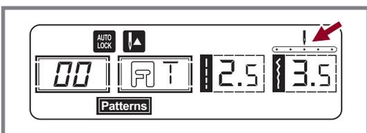
When patterns 00-04 are selected, the needle position is regulated by the stitch width adjustment buttons. Pressing the "-" button (left), will move the needle to the left and pressing the "+" button (right), will move the needle to the right.
