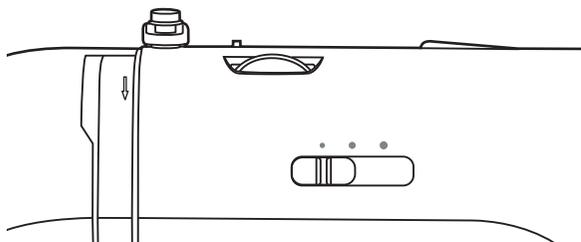
The speed limiting adjustment lever can control the sewing speed. To increase the speed, slide the lever to the right, to decrease the sewing speed, slide the lever to the left.
