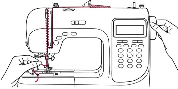
1. Hold the upper thread with the left hand. Turn the handwheel towards you (counterclockwise) lowering, then raising the needle.
