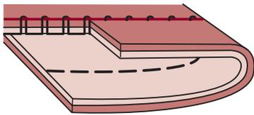
Thread tension is too tight for straight stitch sewing. Turn dial to lower number.
