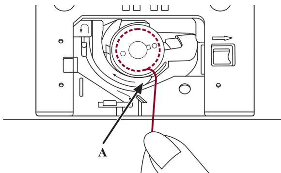
Pull the thread through the slit (A).
