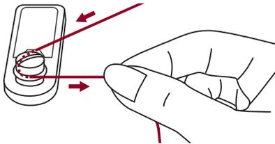
4. Place the thread end through one of the inner holes in the bobbin as illustrated and place empty bobbin on the spindle.
