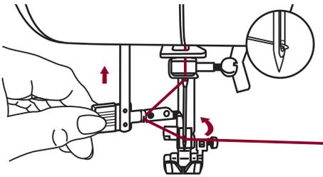
The needle threader automatically turns to the threading position and the hook pin passes through the needle eye.
