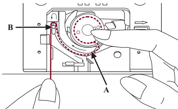
With a finger held gently on top of the bobbin. Draw the thread at the arrow markings into the stitch plate thread guide from (A) to (B).
