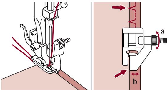
Place the fabric under the foot. Turn the handwheel forwards by hand until the needle swings fully to the left. It should just pierce the fold of the fabric. If it does not, adjust the stitch width accordingly.
