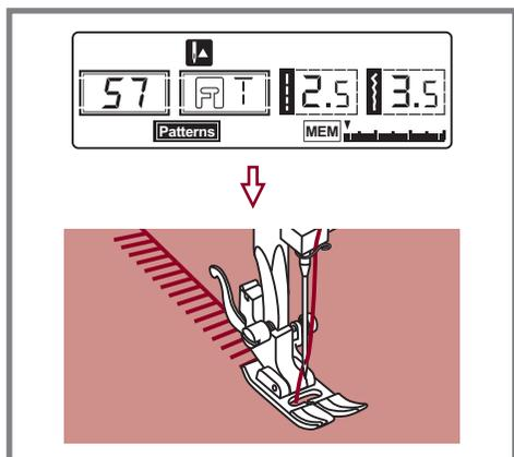
Press foot controller. The machine will start to sew from first entered pattern. On the LCD screen, sewing stitch data is indicated.
