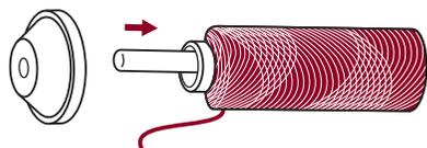
1. Lift up the spool pin. Place the spool of thread on the spool pin so that the thread comes from the front of the spool, then place the spool cap at the end of the spool pin.
