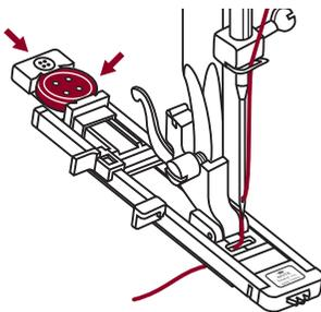
Attach the buttonhole foot, then pull out the button holder plate and insert the button.
