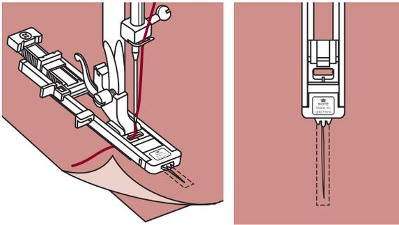
Baste the upper fabric and the under fabric together. Select the needle position. Lower the presser foot over the center of the tear.
