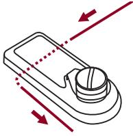
3. Guide the thread around the thread guide pulling the thread through the pre-tension spring as illustrated.
