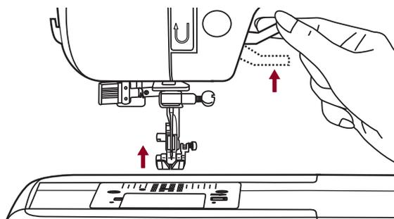
When sewing several layers or thick fabrics, the presser foot can be raised a second stage for easy positioning of the work.
