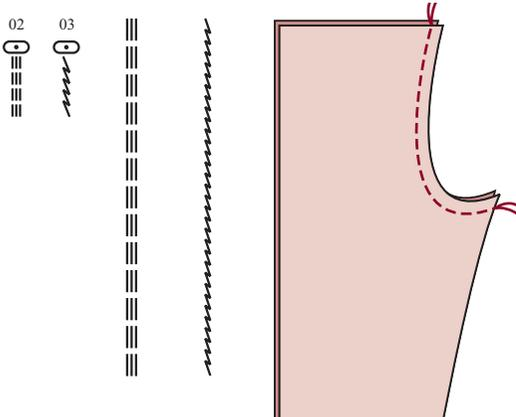
Straight stretch stitch is used to add triple reinforcement to stretch and hardwearing seams.
