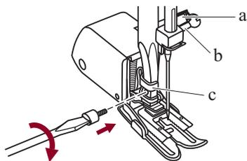
Attach the Walking Foot to the machine as follows:
