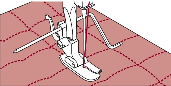
Sew the first row and move over the fabric to sew successive rows with the guide riding along the previous row of stitching.
