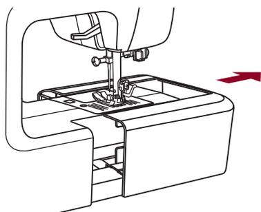
With the sewing table off the machine, the feed dog adjustment lever can be seen on the base in back of the sewing machine.
