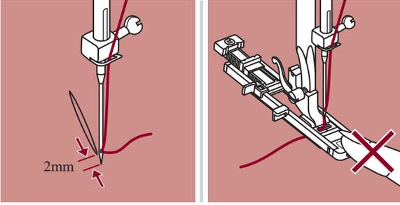
Position the fabric so that the needle is 2mm (1/16 inch) in front of the area to be darned, and then lower the presser foot lever.
