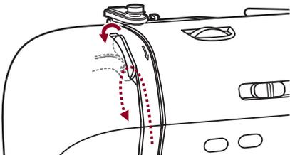
6. At the top of this movement, pass the thread from right to the left through the slotted eye of the take-up lever and then downwards again.
